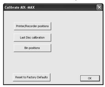
Last Disc calibration and Bin positions will only be necessary if the Autoloader is having trouble picking from the bins. Follow the onscreen prompts to calibrate the bins.
